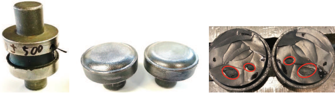
Figure 2: The shear specimen with typical crack initiations (highlighted in red) in the volume of the sliced specimen after one-sided cyclic shear load.
