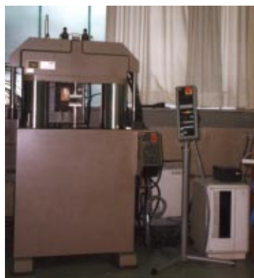
Figure 2: The Servo hydraulic testing machine with clamped test specimen
